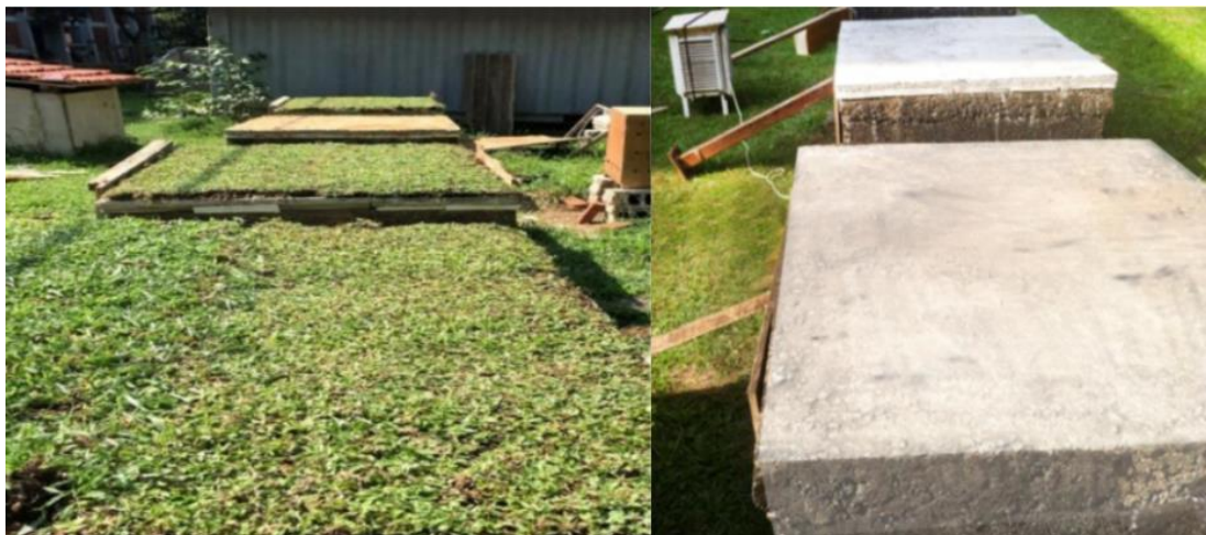
Figure 15, Physical models constructed for thermal performance comparison
