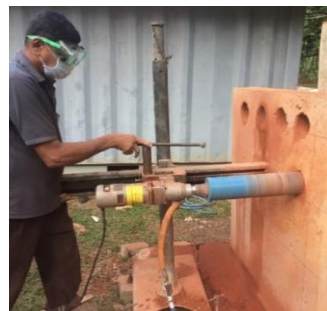
Figure 3, Obtaining MC core samples
