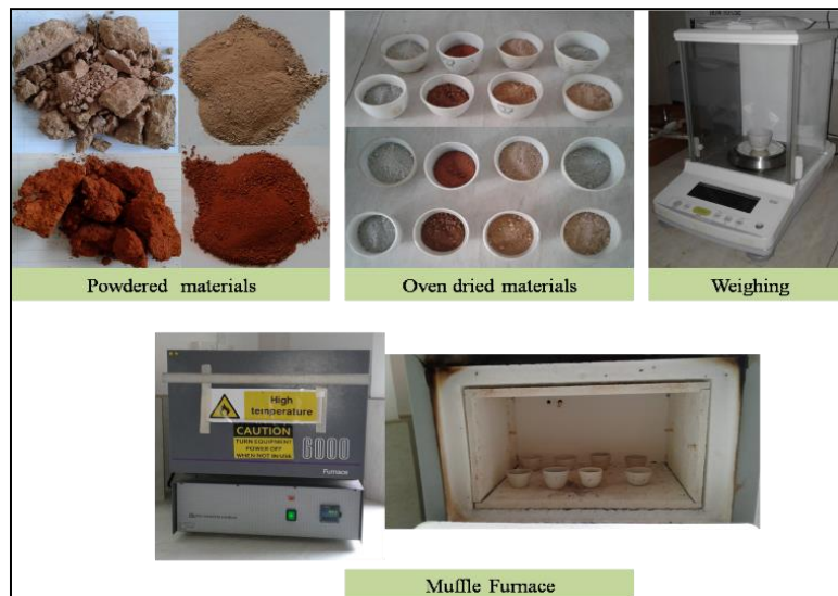
Figure 1, Testing of organic matter content
