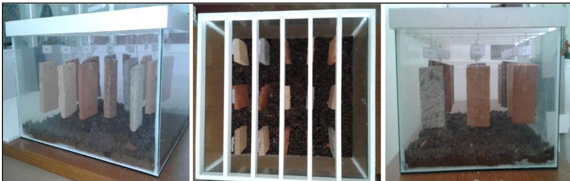
Figure 5, Samples testing in the environmental chamber
