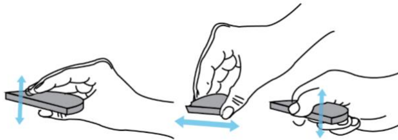
Figure 20: Actual Pinch Grip Applied on the Disk-like Handle (Source: Author)
