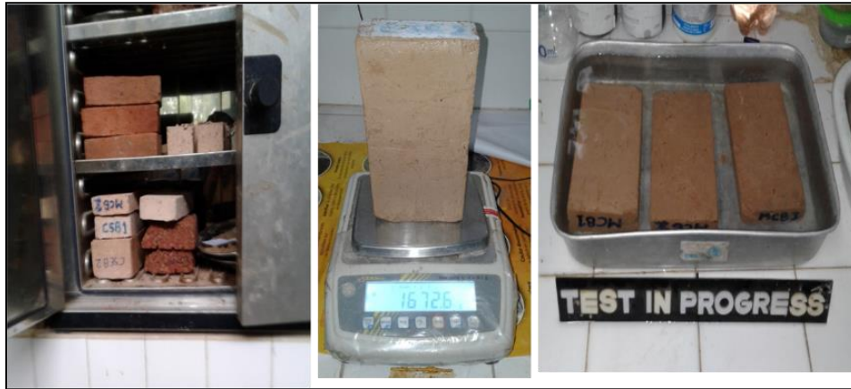
Figure 3, Water absorption test
