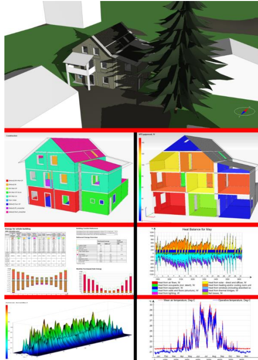
Figure 1. Building performance simulation model with input and some resulting output (Source: Wikipedia)
